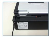
STEP 5— If the Otogram will be stored, transported or not used for an extended period of time, then replace the Connection Port Dust Covers.
