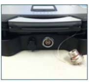
STEP 2 - Connect the Otovest Connector to the Otovest Connection Port.
